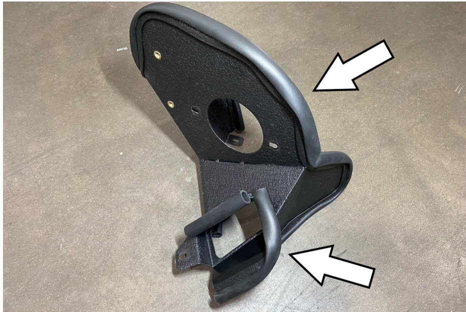
11. Install the provided bubble edge trim onto the HPS upper heat shield in the areas shown.
