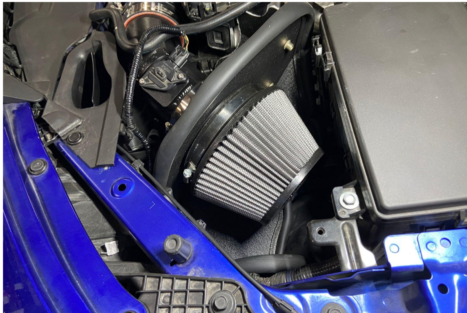
22. Install the provided HPS performance air filter using either a flat head screwdriver or 8mm socket.
