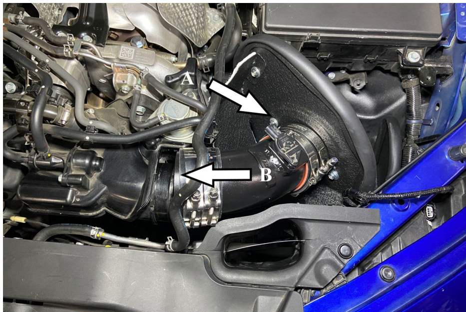
20. Insert the intake pipe onto the velocity stack first (A), then slide the other coupler (B) onto the turbo inlet side. Position the intake pipe into place and use a 10mm socket to tighten all of the T-bolt clamps to 15 in-lb.
