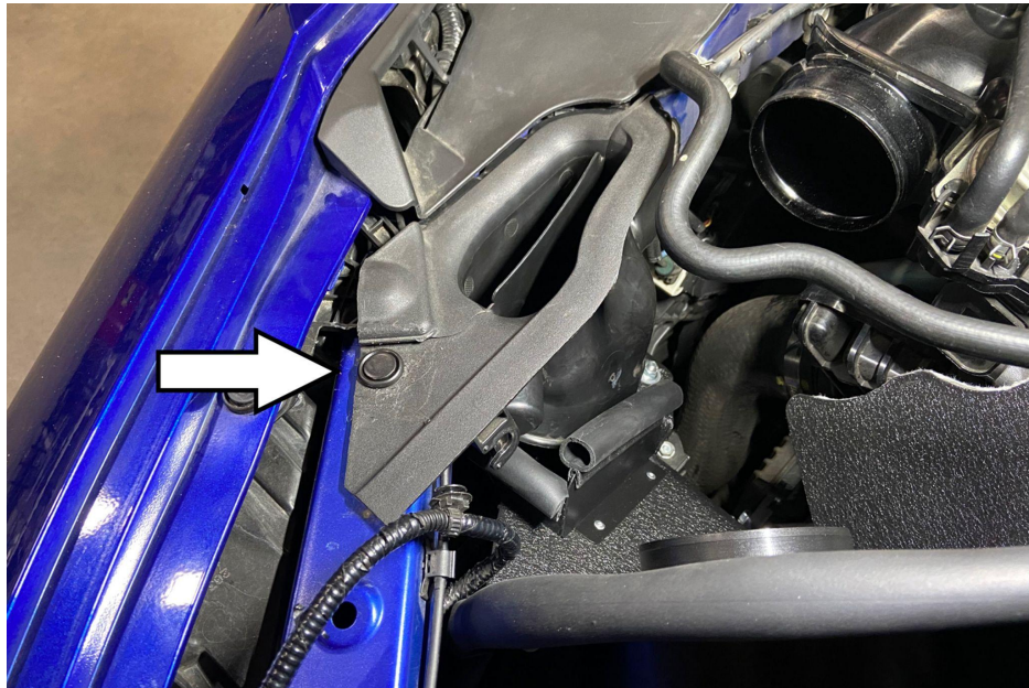
19. Reinstall the factory air duct back into the vehicle.
