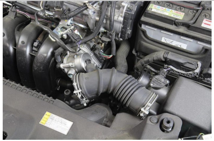
5. Remove the stock intake tube from the vehicle.
