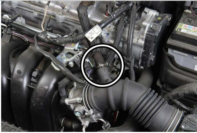
4. Depress the spring clamp and remove the breather hose from the intake tube.
