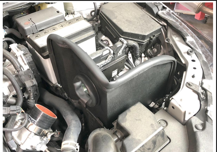
13. Place the heat shield on top of the stock lower air box. Be sure that the heat shield sits to the right of the ears.
