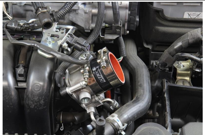
9. Insert the provided silicone coupler along with the t-bolt clamps onto the throttle body.
