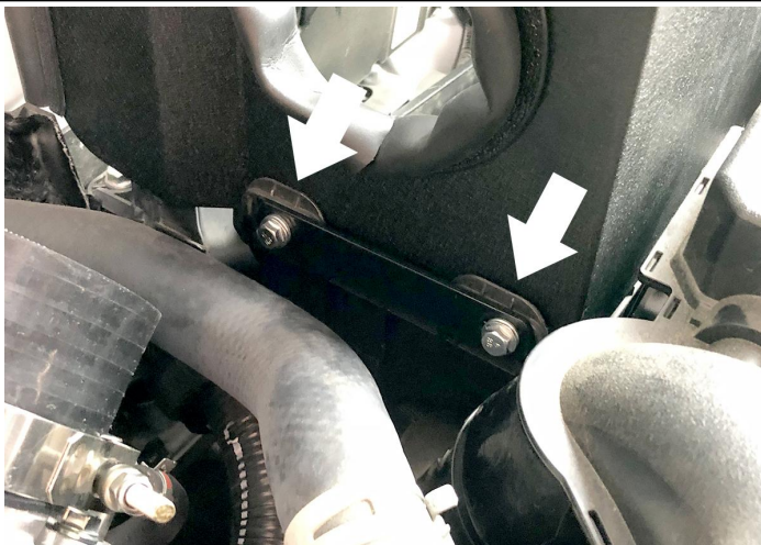
14. Place the flat bracket in front of the ears, then slide in the long bolts along with a washer through the hole.
