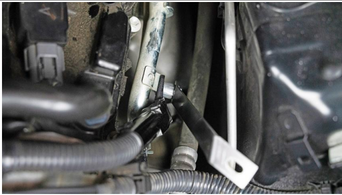
16. Loosley insert the bracket replacing the bolt in step 14.
