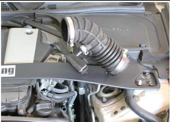
12. Remove the driver side intake hose from the vehicle.
