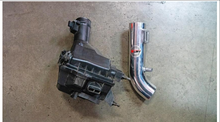
17. Remove the factory Mass air flow sensor and install the sensor onto the HPS intake pipe using our provided M4x8mm Allen bolts.
