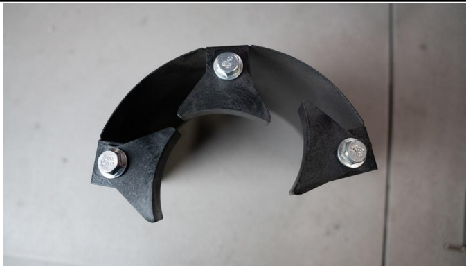
22. Loosely install the heatshield brackets onto the heat shield.
