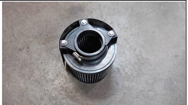
23. Use the provided EMSC-70-90 clamp to secure the heatshield onto the HPS performance air filter.
