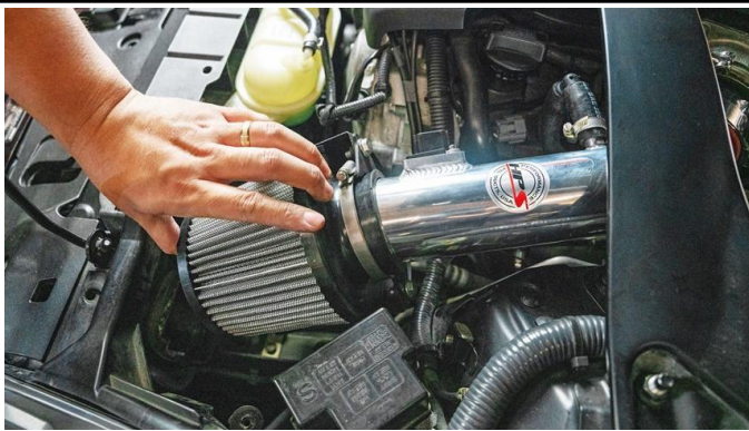
24. Insert and secure the HPS performance air filter along with the heat shield onto the intake pipe.
