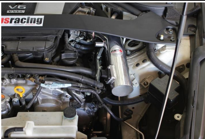
18. Install and secure the HPS intake to the bracket using the provided M6x12mm bolt and washer, then tighten the bracket down once its in position.
