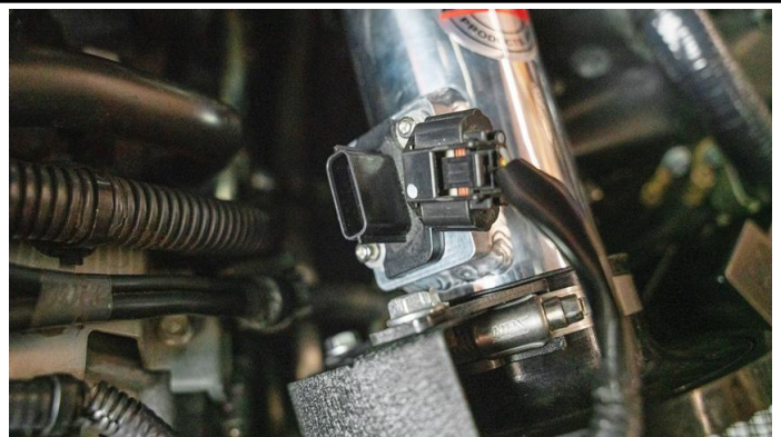
25. Re-connect the MAF sensor harness connector.
