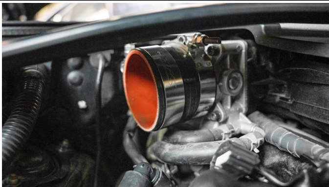
26. Install the silicone coupler along with the provided T-bolt clamps onto the passenger side throttle body.
