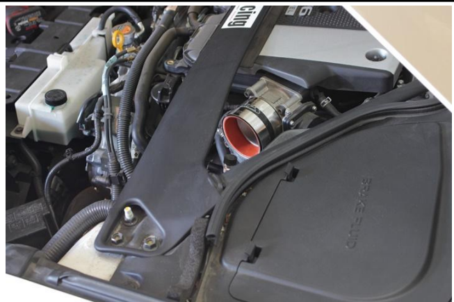
13. Install the silicone coupler along with the provided T-bolt clamps onto the driver side throttle body.
