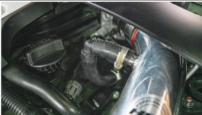
20. Install and secure the EPDM hose onto the intake barb using the provided EMSC- 16-27 clamps.
