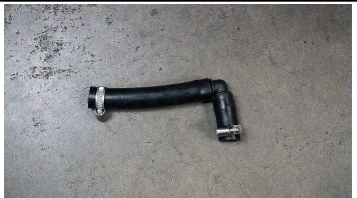
19. Assemble the passenger side breather hose using one of the 5-inch EPDM hose and a 2-inch EPDM along with the provided 90 degree barb.
