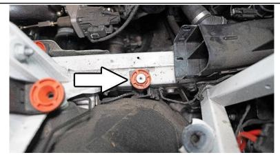
12. Insert the provided M6 bung into the bottom factory heat shield grommet.
