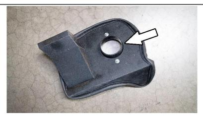
11. Install and secure the provided velocity stack onto the heat shield using the M6 x12mm bolts and washers.
