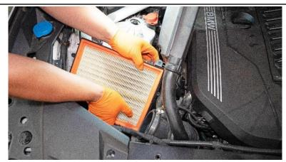
8. Lift up and pop the lower air box from its mounting grommets and disconnect the hose from the turbo inlet housing then carefully remove the assembly from the engine bay.
