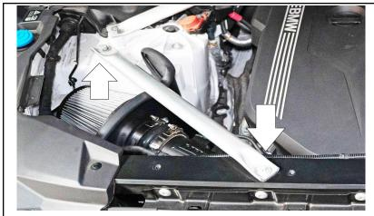
21. Re-install the passenger side strut tower brace into the vehicle.
