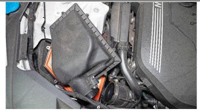
6. Disconnect the upper air box portion from the intake hose and remove it from the vehicle.
