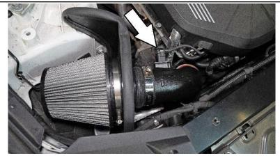
20. Insert and fasten the HPS performance air filter to the velocity stack. Reconnect the sensor.
