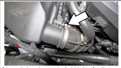
5. Loosen the hose clamp securing the intake hose from the upper air box.
