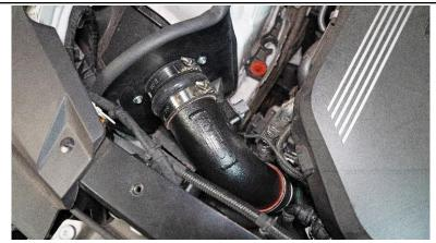
18. Fasten the T-bolt clamp to secure the hump coupler onto the velocity stack.
