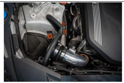
16. Insert the heat shield into the vehicle.
