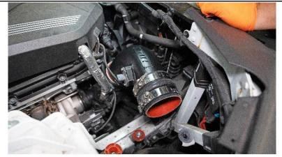
15. Insert the HPS intake into the reducer coupler.
