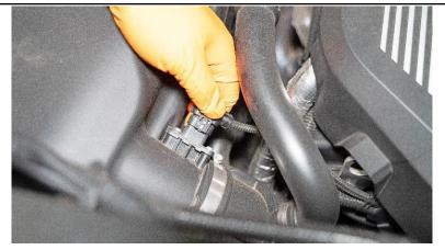
3. Disconnect the sensor electrical harness connector.
