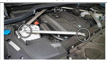
2. Remove the passenger side strut tower brace using a E12 and 18mm socket.
