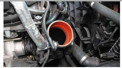
9. Insert the provided reducer coupler along with the embossed clamps onto the turbo inlet housing.
