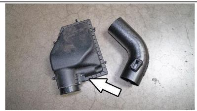
13. Transfer and secure the sensor onto the HPS intake pipe using the provided M4 bolts.
