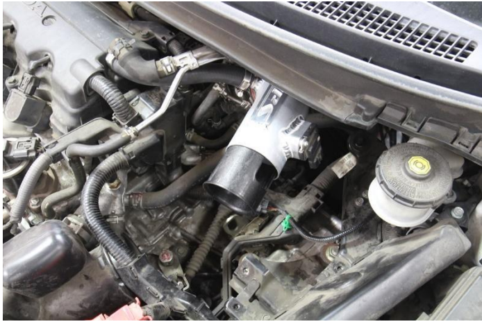
14. Insert the provided 2.75" air straightener into the intake pipe and secure the 16mm EPDM hose onto the intake pipe.
