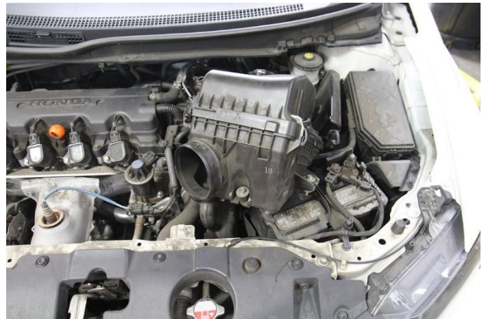
7. Disconnect the air box assembly from the rubber grommet mount and remove the air box assembly along with the intake hose from the vehicle.
