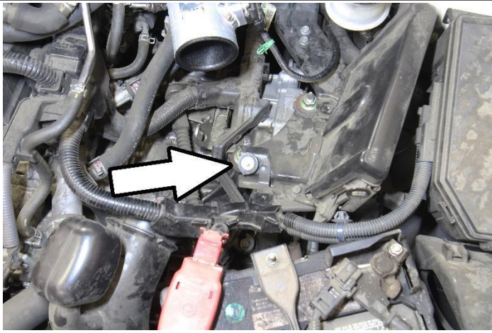
16. Insert and secure the provided 1/2" vibration mount into the factory air box mounting hole.
