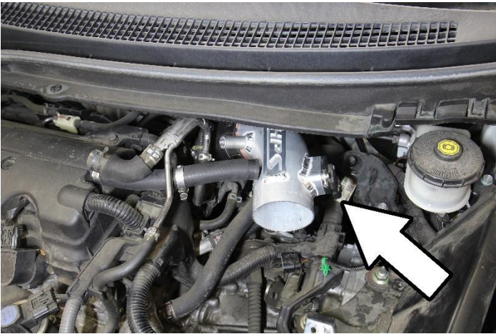
13. Install and secure the factory MAF sensor onto the HPS intake pipe using the provided M4 bolts, then insert the intake pipe into the throttle body coupler.
