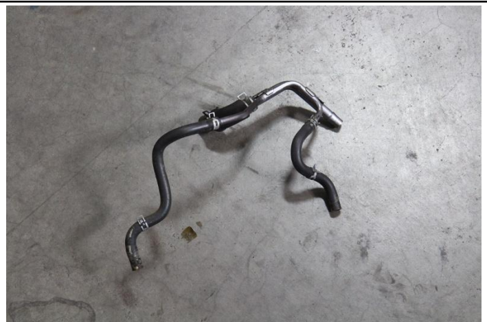
9. Remove the throttle body hoses and the breather hose hardlines from the vehicle.
