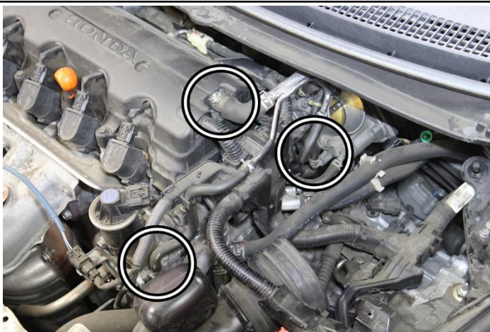
8. Depress the retaining clamps securing the breather hose from the valve cover and the throttle body coolant hoses. *Be sure to use a bag to catch any residual coolant from the throttle body hoses.
