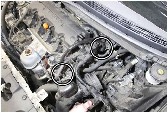
10. Install the provided 8mm heater hose line along with the two FIC-12 clamps to replace the factory throttle body hoses.
