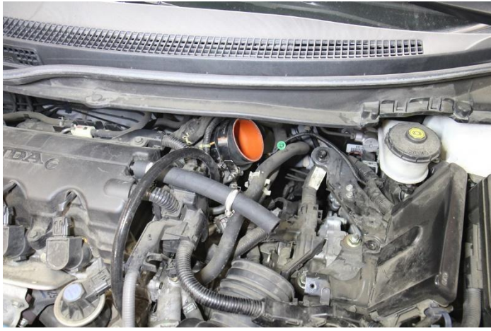
12. Insert the reducer coupler along with the provided T-bolt clamps onto the throttle body. Remove the factory air duct hose from the air duct tube.
