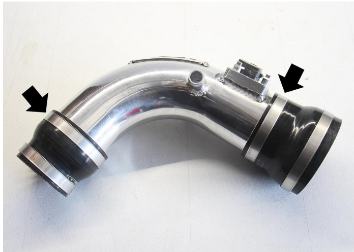
12. Install the silicone reducers onto the intake pipe as shown. Tighten the hose clamps onto the intake pipe.
