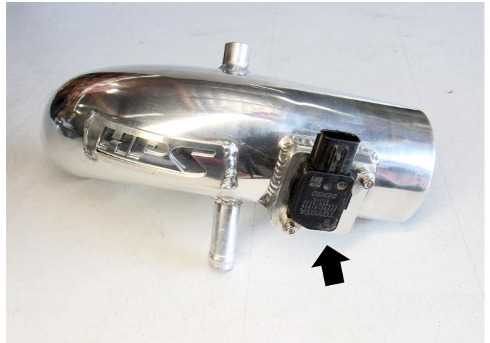
11. Transfer the MAF sensor from the stock air box onto the HPS intake pipe and secure with the M4 screws provided.
