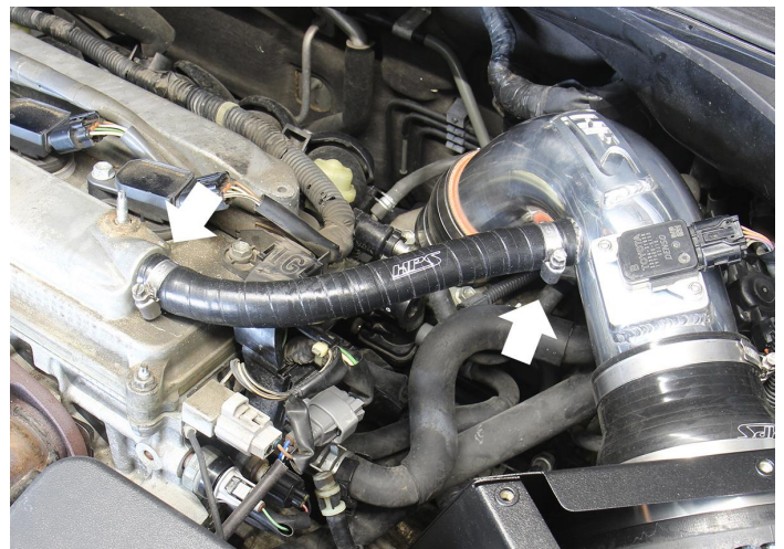
21. Connect the provided EPDM hose in between the valve cover and intake pipe then secure the hose using the provided hose clamps.
