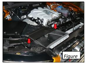
Disconnect the factory rubber hose and plastic fitting from the intake tube, at arrows in **Figure 3**.
