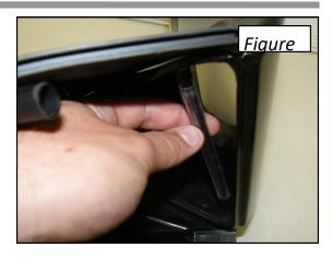
Remove the carbon fiber inlet duct and use the included drill bit to drill the lower air box at the previously marked locations on the tabs.
