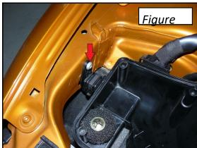
With the bracket removed pull up on the lower air box to gain access to the air pump hose below.
