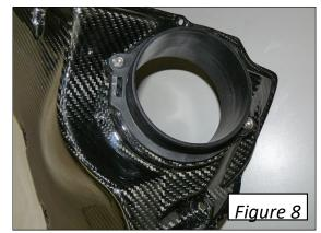
Install the AWE S-FLO Filter onto the AWE Carbon Air Box Lid using the same hardware that attached it to the OE air box lid.
