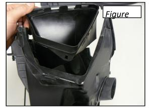
To remove the lower air box, remove the T30 screw from the black plastic mounting bracket.
