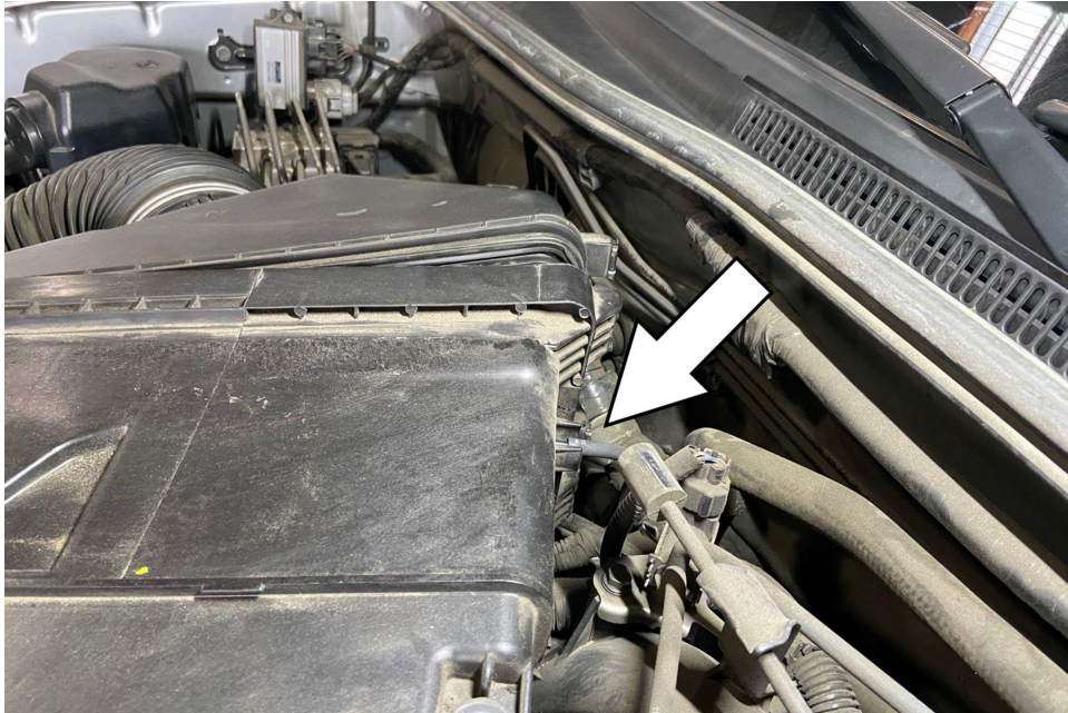
6. Disconnect the vacuum hose from the back side of the air box assembly.
