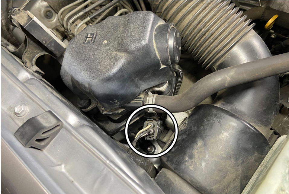
9. Disconnect the air pump electrical harness connector.
