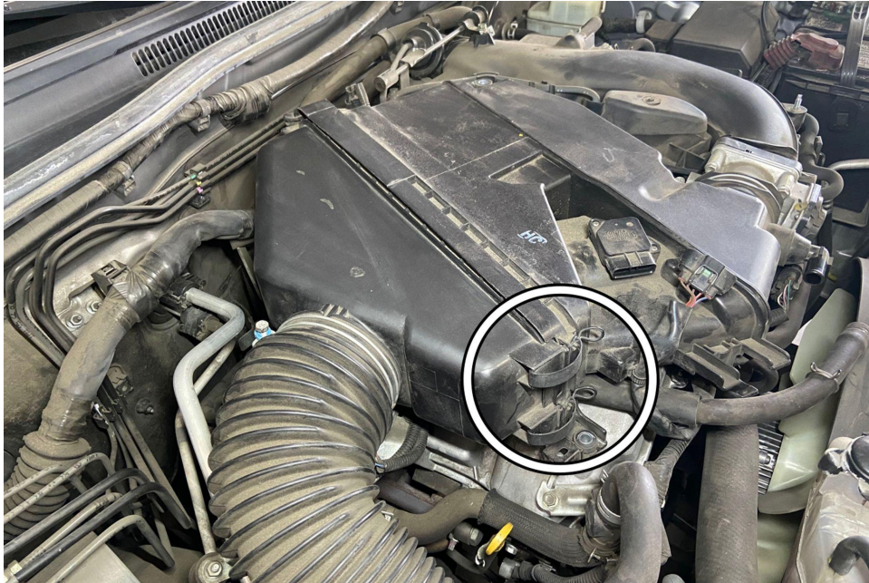
5. Loosen the retaining clips securing the air filter box.
