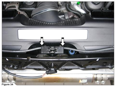
! WARNING: direct and secure (use additional plastic ties) the rubber hoses in such a way, that they don't touch any hot or moving parts of the vehicle!
