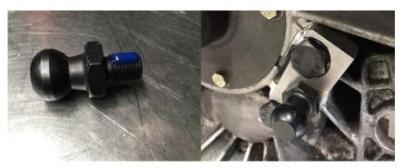
5) Using high temperature bearing grease, lubricate all the points of contact on the fork. This includes where it contacts the bearing carrier, push rod and pivot ball.
