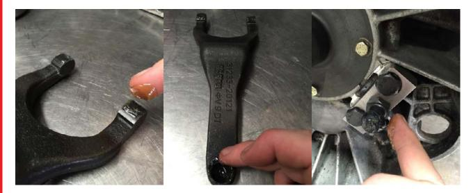
6) Install the release bearing clip onto the release bearing carrier. This clip only fits in one direction with the small tab on the bearing carrier holding the clip in place.
