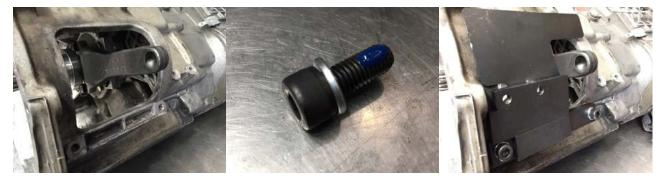
10) Use M8X1.25X20 bolts with spring washers to mount the slave cylinder in place on the adapter plate. Then install the new braided clutch line to the slave
