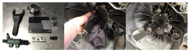
3) Use the pivot ball bracket and fix it to the transmission using the M10X1.25X20 bolts supplied along with the spring washers and thread lock. Ensure that the bracket is mounted in the correct orientation with the small chamfered edge facing upward. Torque the bolts up to 50Nm.
