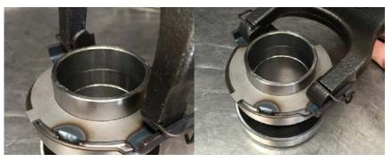
8) Lubricate the nosecone on the transmission and slide the release bearing and fork into place. Clip the clutch fork onto the pivot ball with a firm push.
