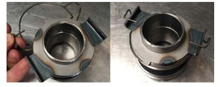
7) Connect the clutch fork to the release bearing carrier by tilting the fork under the clip so the clip sits in the grooves of the fork.
