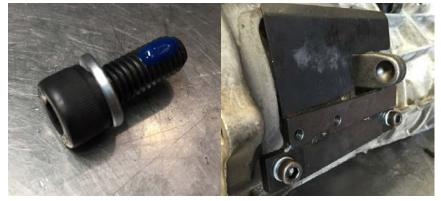
10) Use M8X1.25X20 bolts with spring washers to mount the slave cylinder in place on the adapter plate. Then install the new braided clutch line to the slave.
