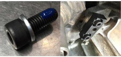
4) Use the new pivot ball supplied and install it onto the pivot ball bracket using thread lock. Torque it up to 70Nm.
