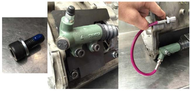
11) With the clutch mounted to the engine the transmission can be carefully mounted to the engine. Connect up the braided line to the existing hard line.
