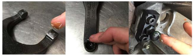
6) Install the release bearing clip onto the release bearing clip. This clip only fits in one direction with the small tab on the bearing carrier holding the clip in place.
