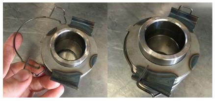
7) Connect the clutch fork to the release bearing carrier by tilting the fork under the clip so the clip sits in the grooves of the fork.
