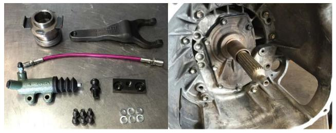
3) Use the new pivot ball bracket and fix it to the transmission using the M8X1.25X20 bolts supplied along with the spring washers and thread lock. Ensure that the bracket is mounted in the correct orientation with the milled out mounting bolt holes toward the input shaft. Torque the bolts up to 32Nm.
