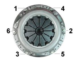
The bolts need to be tightened in a "star" type formation. See picture. Please refer to manufactures workshop manual for recommended torques.
