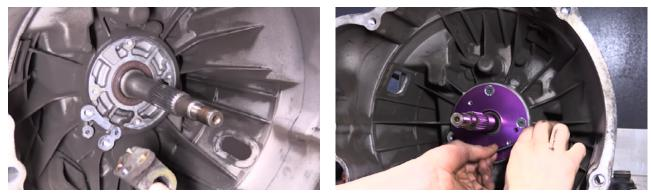
Step 5:Clean the mounting surface at the back of the bellhousing.
