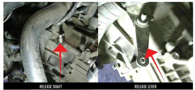
Caution: If the gearbox is installed without doing this step the release bearing can separate from the clutch fork
