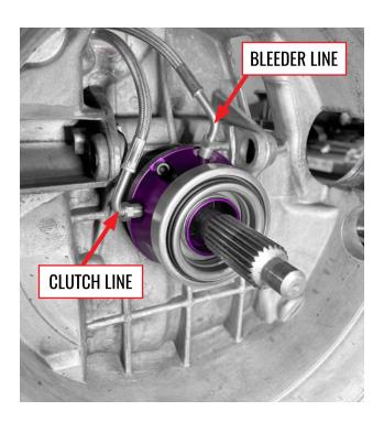
7. Before assembling the remainder of the vehicle, check for full release of the clutch. Place the transmission into gear and have one person holding the clutch, while another person rotates the drive shafts to ensure that the clutch is releasing. Once confident that the clutch has adequate release, assemble the rest of the vehicle and test drive.
