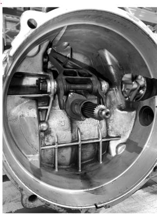
2. Apply a small amount of thread retaining compound to the supplied countersunk M6 bolts and fit the Xtreme CSC spacer, with the straight cut edges facing the bottom of the bellhousing. Torque the bolts to 10Nm/8ft.lbs. Install the steel shim onto the spacer to locate the base of the CSC.
