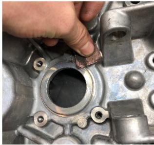
3. Mount the release bearing adapter to the transmission & use a small amount of thread retaining compound on the 4 counter sunk bolts to holt it in place. Torque them to 10Nm/8ft.lbs.
