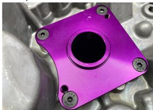
4. Install the small steel shim onto the adapter to centrally locate the body of the slave.
