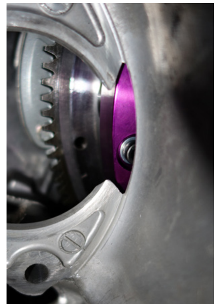
Clearance on clutch can be seen from outside the bellhousing.
