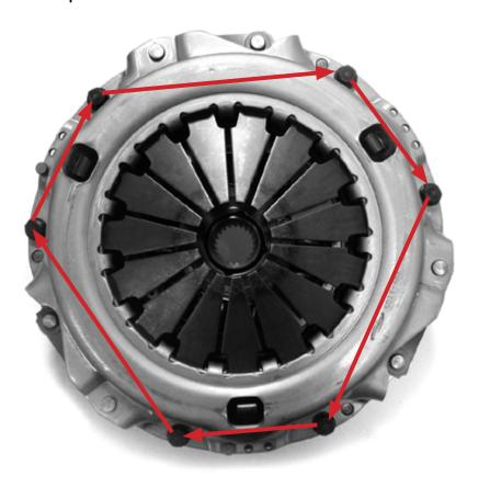
Tighten all bolts  $\frac{1}{2}$  a turn at a time, following the sequence and repeat until tight. Finally, torque the bolts to the manufacturer's specification.
