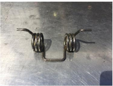
Spring removed from pedal assembly.
