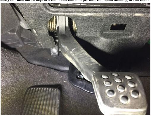
Remove the panel above the pedals to allow access to the spring.
