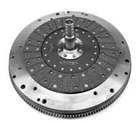
2b. Fit the intermediate plate over the dowels on the flywheel, making sure to line up the index marks. The second disc can then be fitted over the aligning tool, following the labelling on the disc for the correct orientation. If there is no labelling on the disc, ensure it is sitting flush on the intermediate plate and has clearance between the hubs.
