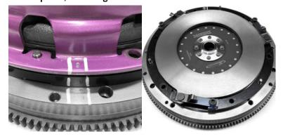
2. Remove the intermediate plate from the flywheel by using a flat blade screwdriver under the cutout sections at the dowels. The bottom disc can now be removed. **Do not lever under the intermediate plate straps or loosen the bolts holding the straps on the intermediate plate.**
