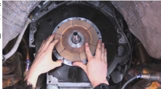
9. Install the main pressure plate casting into the alloy hat with the fulcrum ring facing toward the diaphragm. Slide this over the alignment tool and locate the alloy cover on the flywheel.
