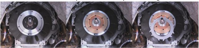
8. Select the next friction disc and take note of the orientation of the hub before installing it on the alignment tool. Be sure to check that the hubs do not interfere with one another in the installation order.
