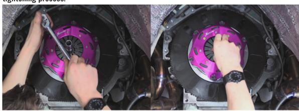
11. Finally, torque the bolts to 31Ft.lbs/41Nm.
