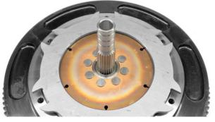
3. Place the final disc onto the flywheel, followed by the pressure plate casting, making sure that the flat friction surface is against the ceramic facing. Ensure the "teeth" of the intermediate plates and pressure plate casting align so that the pressure plate bolt holes are in the gaps, circled in red.
