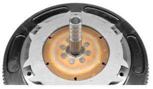
2. Place the second disc onto the flywheel, followed by the second intermediate plate. Note that for quad disc kits, there will be an additional disc & intermediate plate before the final disc and pressure plate casting.
