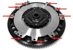
4) Install the top friction disc on the intermediate plate. Ensure on the sprung version that the outer ring is facing upward to mate correctly to the driving teeth on the bottom disc. On a rigid hub version, visually check that there is clearance between the hubs of the top and bottom discs.
