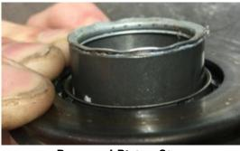
**Damaged Piston Stop**
