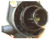
Off Axis Wear On Guide Tube
