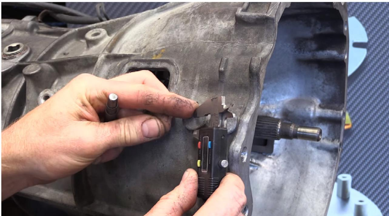
2. Carefully mark the centre of the casting on the bellhousing where the new slave will mount.
