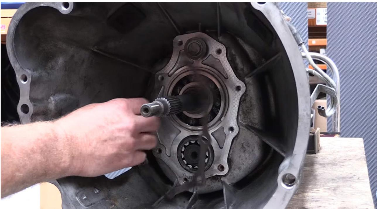
8. Remove front cover of the transmission by undoing all of the bolts & then remove the front cover gasket.
