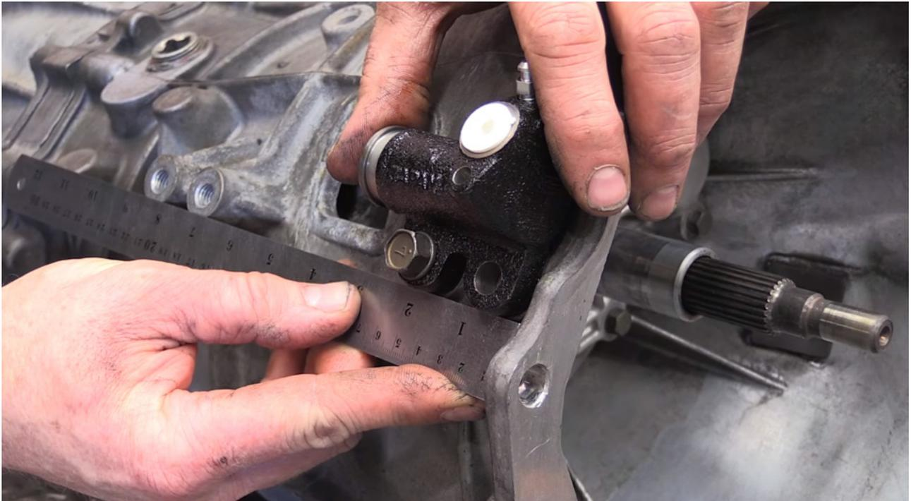
5. Mount the slave on the casting with this one bolt hole and align the slave to the centre of the fork window
