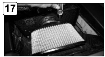
Install filter and tighten using 5/16" nut driver. Re-install engine cover. Re-connect battery terminals.
