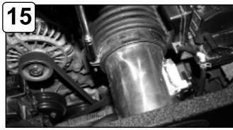
Tighten clamp using 10mm socket or wrench. Re-connect MAF sensor harness.
