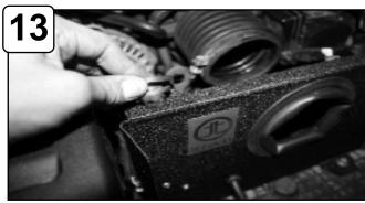
Remove OE grommets from air box and install to hole cut outs on top of housing.
