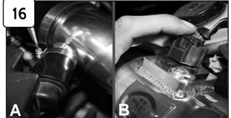
A)Attach 05-01043 coupling from the crank case port on the intake, to the stock plastic vacuum port. B)Re-connect MAF sensor harness.
