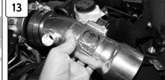
Install intake assembly and position tab to isolation mount. Do not tighten.
