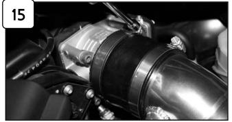
Tighten all clamps using 5/16" nut driver.
