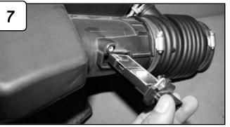
Remove MAF sensor using phillips screwdriver.
