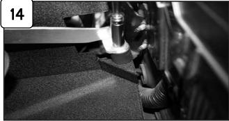
Tighten tab using provided Flat washer, wavy washer and nut.
