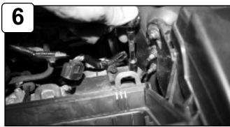
With 10mm socket or wrench loosen the bolt securing bottom half of air box. Carefully remove stock air box assembly out of vehicle.
