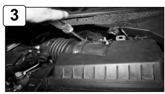
With 5/16" nut driver loosen clamps on stock intake.
