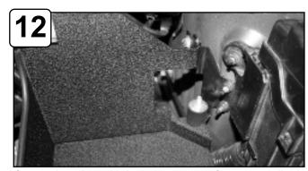
Secure housing with isolation mount. Secure small tab using M6 screw, wavy washer and nut. Tighten all screws and bolts using 10mm socket or wrench.
