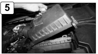
Remove upper half of air box and stock tube w/ carbon attachment assembly.
