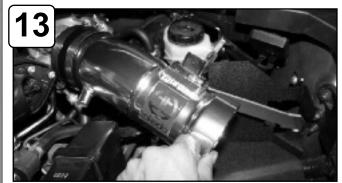
Install intake tube assembly and position tab to isolation mount. Do not tighten.
