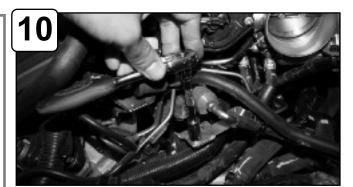
With 10mm socket or wrench loosen bolt on engine.
