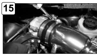
Tighten all clamps using 5/16" nut driver.
