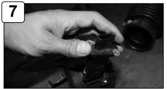
Remove MAF sensor using phillips screwdriver.
