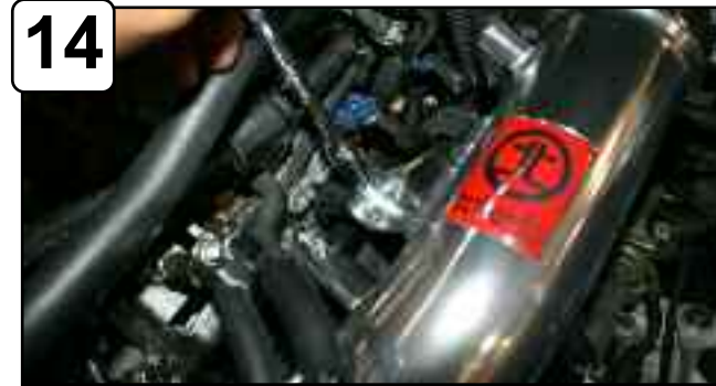
14 Secure tab on tube to engine. Tighten using provided screw and flat washer.
