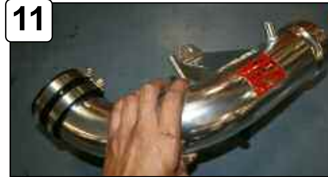
11 Attach coupler to tube using clamps provided. Do not tighten. Install grommet to hole on tube.
