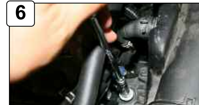
With 10mm socket or wrench loosen clamp on throttle body. With 10mm socket or wrench loosen the 3 bolts holding in air box.
