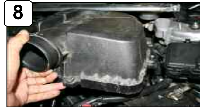
Remove upper half of air box assembly.
