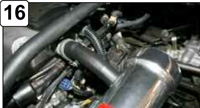
16 Reinstall the crank case line using the provided 5/8" hose.
