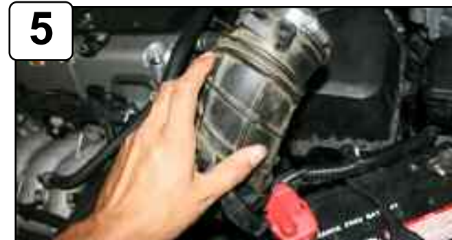
Remove stock intake tube.
