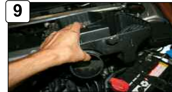
Remove bottom half of air box assembly.
