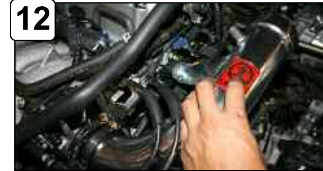
12 Install intake assembly and position. Do not tighten.
