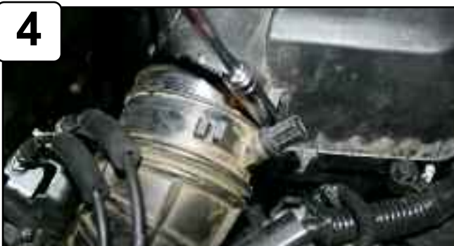
Loosen clamp on air box using 10mm socket or wrench and disconnect temp sensor harness.
