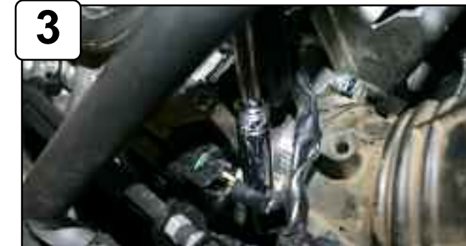
With 10mm socket or wrench loosen clamp on throttle body.
