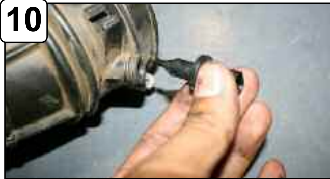
10 Remove temp sensor from stock intake tube.
