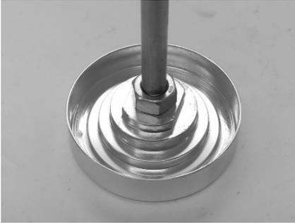
The upper spring support is stepped to accommodate the inner, middle and outer springs. Each spring should be seated on their respective step.
