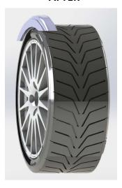
A1 \_\_\_\_ mm - A2 \_\_\_\_ mm - 2mm (clearence guarantee) = \_\_\_\_ mm wheel spacer (example: (A1) 27mm - (A2) 5mm - 2mm = 20mm ST wheel spacer)
