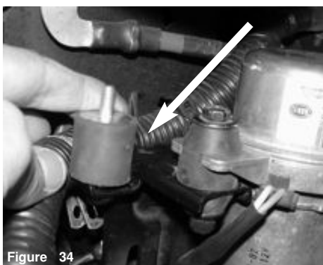
Figure 34 Loosen the bolt holding the harness bracket, and replace with provided M6 vibra mount.
