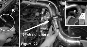
A)Attach the 3" straight hose with clamps to the primary intake tube. Now install the secondary tube and connect to tighten all clamps using 8mm nut driver. Tighten and the primary tube. Do not tighten.B)Connect the crankcase secure the vibramount using 10mm socket or wrench. line to the engine fitting.
