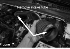
Carefully lift up and remove the stock intake tube from the
