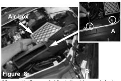
A)Loosen the 2 screws holding in the airbox snorkel using 8mm nut driver or socket.
