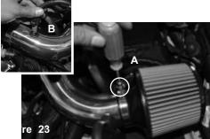
A)Install the air filter. Position the intake for the best fit, B)Install the temp sensor, make sure harness is connected. Re-install the engine cover. Connect the battery terminals
