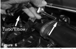
Loosen the clamp on the plastic turbo elbow. Remove the stock intake tube from the turbo elbow. Un-clip upper half of air box.
