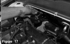
nstall the step hose to the turbo with clamps provided.
