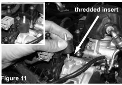
Install the vibramount to the thredded insert from step 5. Secure and tighten.
