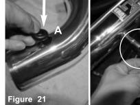
A)Install the grommet to the hole in the secondary tube. B)Connect the vacuum line to the fitting on primary tube.
