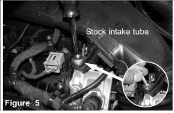
Locate the screw holding in the upper half of the stock intake tube. Loosen using 8mm nut driver or socket. Remove the screw.
