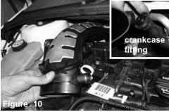
Loosen the clamp on the turbo side, remove the plastic turbo elbow. Disconnect the crankcase line.
