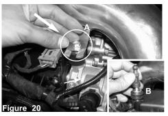
A)Install the primary intake tube and secure to the turbo and bracket to the vibramount. Secure using provided m6 nut and fender washer. B)Re-install the fitting from step 9, this will allow for the engine cover install.
