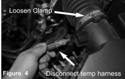
Loosen the clamp on the upper part of the air-box. Disconnect temperature sensor harness. Turn and pull the temperature sensor out of tube.
