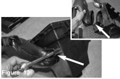
Loosen the screw holding in the factory scoop on the air box. This will be used in the new intake kit.
