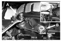
A) Loosen the 8mm screw holding in the plastic turbo elbow. Remove the screw. B)Now loosen the engine cover fitting using 12mm wrench. Remove and save fitting and grommet with spacer for later install.
