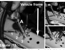
A) Loosen the 3rd ground strap. Save bolt for later install. B) Loosen the 1st ground strap.
