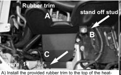
shield, notch in corners with knife or scissors for cleaner installation. B) Install the provided m6 stand off stud to factory grommet air box position. C) Install the heat shield and position bracket to stand off stud, and thredded insert from step 12. Secure using factory screw. Secure the stand off stud using provided m6 nut and washer.
