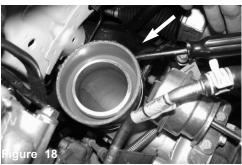
side in a spot allowing for easy access when you tighten 11. Secure and make sure the seal seats and the clip the clamp.
