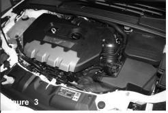
Stock air box assembly shown in this picture. Disconnect battery before the install. Remove the engine cover.
