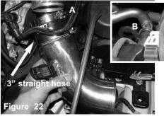
A)Attach the 3" straight hose with clamps to the primary and bracket to the vibramount. Secure using provided m6 intake tube. Now install the secondary tube and connect to en all clamps using 8mm nut driver. Tighten and secure the primary tube. Do not tighten.B)Connect the crankcase line to the engine fitting from step 11 &19.
