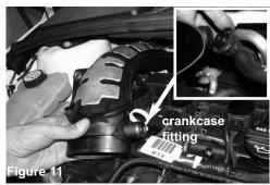
Loosen the clamp on the turbo side, remove the plastic turbo elbow. Disconnect the sensor-harness line. Disconnect the crankcase line.
