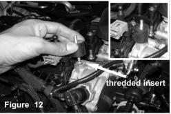
Install the vibramount to the thredded insert from step 5. Secure and tighten.
