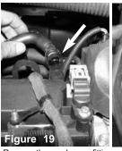
clicks. Lubricate inside of fitting, rotate and position for easier installation
