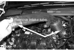
Carefully lift up and remove the stock intake tube from the
