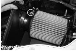
Install the air filter. Position the intake for the best fit, tightthe vibramount using 10mm socket or wrench. Connect the temp sensor. Re-install the engine cover. Connect the battery terminals.
