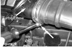
Loosen the clamp on the plastic turbo elbow. Remove the stock intake tube from the turbo elbow.
