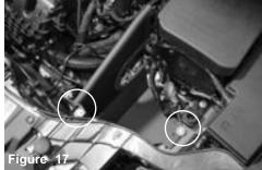
Once fitted properly, secure and tighten both screws using 10mm socket and wrench.
