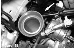
Install the step hose to the turbo with clamps provided. Tighten the clamp on the turbo only. Place clamp on the 3" 11. Secure and make sure the seal seats and the clip side in a spot allowing for easy access when you tighten
