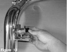
Figure A: Mount the green VAD switching valve onto the bracket on the intake pipe. Re-use the 10mm nut. This VAD switching valve will no longer be used but will remain connected to the ECM to avoid any possible CEL's
