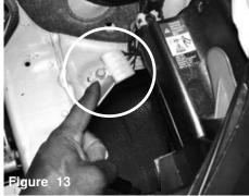
Remove the 10mm bolt on the grounding junction. This grounding junction will be relocated in figure 14
