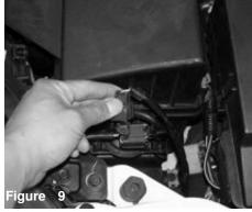
Temperarely disconnect the green harness from the VAD switching valve located on the right side of the factory air box assembly
