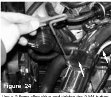
Use a 2.5mm allen drive and tighten the 2-M4 buttonhead screw onto the MAF sensor.
