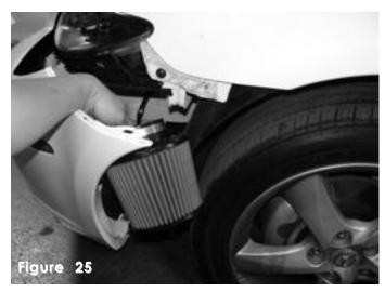
Align the filter to the end of the intake and push the filter over the intake end until the intake has butted up against the filter stops .
