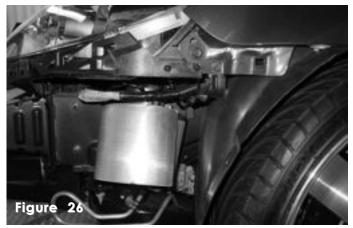
Place the heatshield over the filter and tighten the calmp on the filter.
