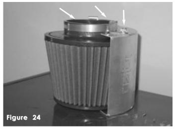
Place 3 - 5/15 flanged bolts and 3 composit HS bracket onto the base of the heatshield and then place heatshield onto the filter base.
