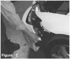
Remove someof the plastic clips and screws securing the drivers side bumper to the fender and radiator shroud. Pull back on bumper to access the intake resonator.
