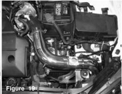
The intake pipe is now in the 45 degree hose and on the vibramount.
