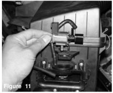
Remove the green VAD switching valve from the air box assembly
