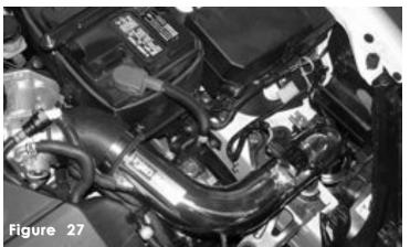
Congratulations! You have just completed the installation of this cold air intake system. Periodically, check the fitment of this intake system to avoid shifting of the intake that may damage the intake from rubbing and banging to other metal parts.
