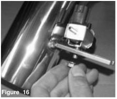
With the filter end of the intake facing down, place the solenoid on top of the intake bracket and use the same nut to fasten the solenoid to the intake bracket.
