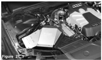
Position for the best possible fit and check for clearance. Re-adjust if necessary.
