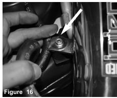
Position for best fit, locate the natural position for the bracket to fit, check filter clearance. Tighten both nuts on brackets using 10mm socket or wrench.
