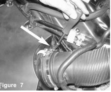
Loosen all the screws holding in the upper part of the air box.
