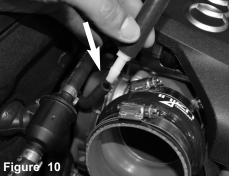
Now attach the coupler extension to the factory vacuum line. Install the 3" hump hose with clamps to the throttle body. Tighten the clamp on the throttle body only.
