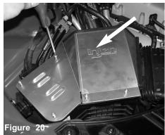
Install the engine cover to the top of the air box, and secure using provided corse screws and tighten using T25 torx screw driver.
