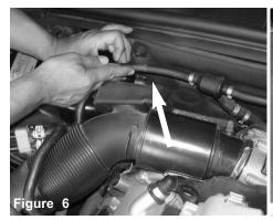
Pull back the vacuum line from the intake tube.
