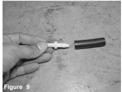
With provided coupler, connect to the 8mm hose. This will be an extension to the intake tube.
