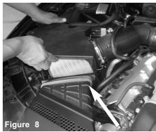
With all lines pulled away from the stock intake system, lift up and remove the stock intake system.
