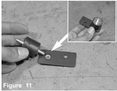
Now install the vibramount to the provided bracket insert. Secure and tighten
