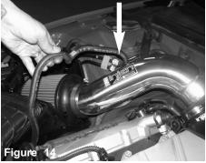
Install the intake tube and position the intake system to the throttle body hose.
