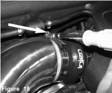
Rotate the intake system if needed for clearance of the filter. Position for the best fit and tighten using 8mm nut driver.
