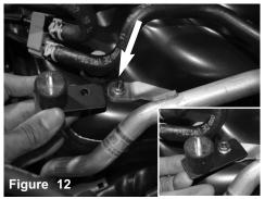
Locate on the strut tower the M6 thredded insert holding the A/C line. Attach the offset side of the bracket to the fitting. Do not tighten.
