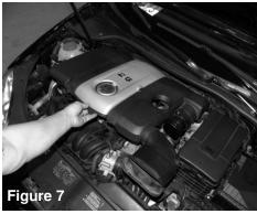
Firmly lift up on the air box/engine cover and remove from the engine bay
