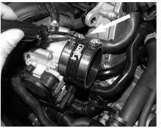
Install the straight hose with clamps to the throttle body. Tightent the clamp on throttle body only using 8mm nut driver.
