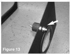
Install the provided vibra mount to the heat shield with vibra mount closes to the engine. Secure using provided m6 nut.
