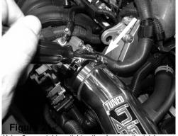
Using 8mm nut driver, tighten the clamp on the intake
