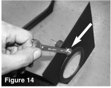
Tighten using 10mm wrench.
