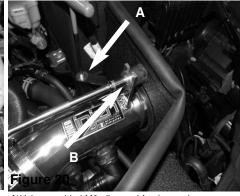
A)Using provided M6 allen and fender washer, secure and tighten the tab on heat shield. B)Position the best fit and tighten the tab on intake tube using 10mm socket or wrench.
