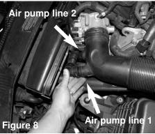
Locate the two air pump lines connect to the throttle body air duct. First disconnect the larger one by firmly pressing on the two release tabs and pulling out and remove the lines.
