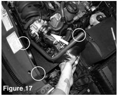
Install the intake assembly into the vehicle and position the intake tube to the throttle body. Position the heat shied to the the tabs from step 10.
