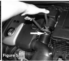
Use a channel lock plier to loosen the pressure clamp on the air air box
