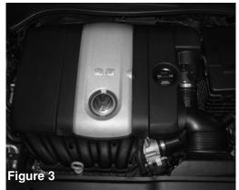
Picture of factory air intake system
