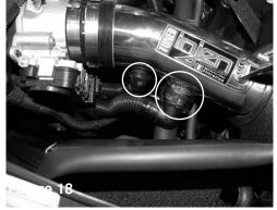
Connect the 2 pump lines to the intake tube fittings. Light With the factory screws lubrication can be put to the inside of the fittings for easier tighten the heat shield.
