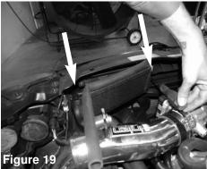
With the factory screws from step 10, secure and tighten the heat shield
