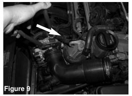
Use a channel lock plier to loosen the pressure clamp on the throttle body and remove the plastic air duct from the throttle body.
