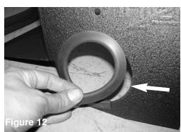
Attach the vinyl trim to the inside of heat shield hole cut out for the intake tube.
