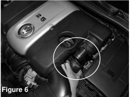
With the pressure clamp loose pull the air duct off the air box
