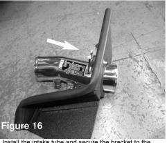
Install the intake tube and secure the bracket to the vibra mount on heat shield using provided fender washer and m6 nut
