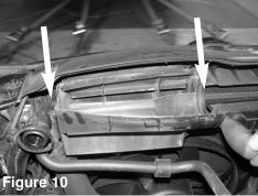
WithT25 torx bit loosen the 2 screws holding in the factory ram scoop and remove. Save screws for later install.
