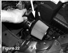
Now install the air filter to the intake tube and tighten using 8mm nut driver.
