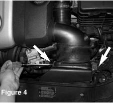
Use a T20 torx screw driver and remove the two torx screws holding the front air box inlet.
