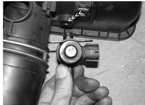
Once the m6 bolt has been removed, continue to pull the OBD sensor from the air box port hole.
