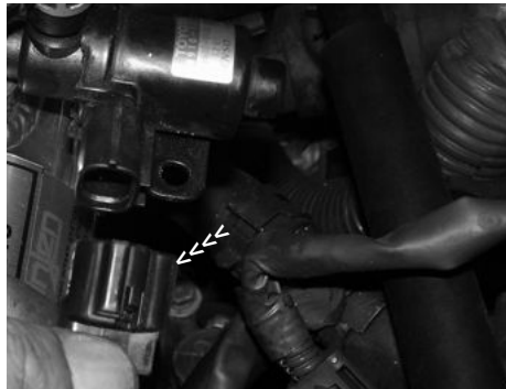
Prior to installing the OBD sensor, connect the harness clip to the OBD sensor as shown above.
