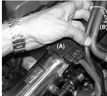
The harness has been connected to the mass air flow sensor (A). Use the zip tie to hold the two vacuum lines together and safe from any moving parts (B).
