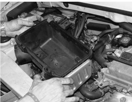
Unscrew the bolts that hold the air intake box in place. Pull the lower intake box from the engine compartment.
