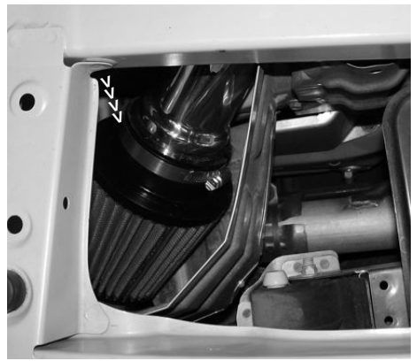
Once the intake has been butted up to the filter stops, continue to tighten the filter neck clamp.
