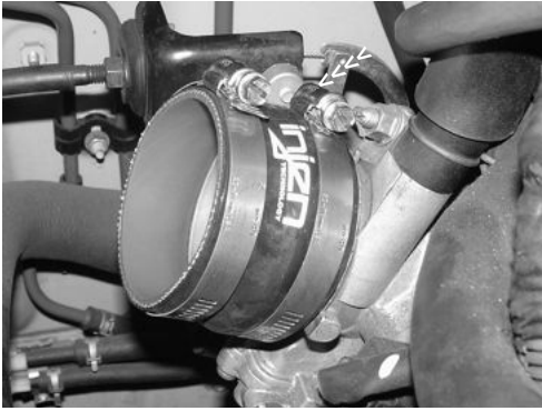
Press the 2 3/4" straight hose over the throttle body. Use two power-bands on the hose and tighten the band on the throttle body side for now.
