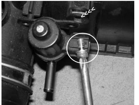
Removing the OBD sensor from the stock air intake box- Unscrew the m6 bolt that holds the OBD to the air box.
