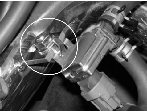
Use the m8 flange nut and bolt to attach the vacuum switching valve to the intake bracket.
