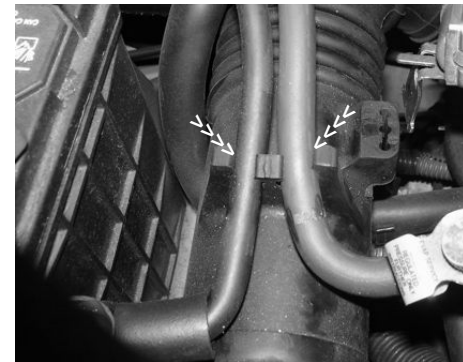
The two vacuum lines are pulled from the saddles built into the rubber intake duct.
