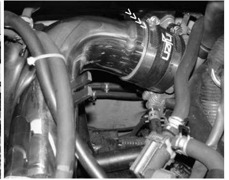
The top end of the intake is pressed into the throttle body straight hose as shown above. Align the intake bracket on the vibra-mount prior to tightening the power-band.
