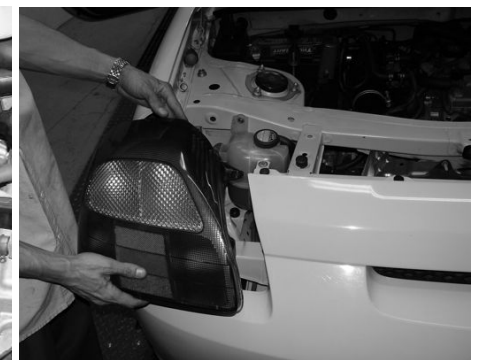
In order to install the filter, the rear tail light will have to be removed.
