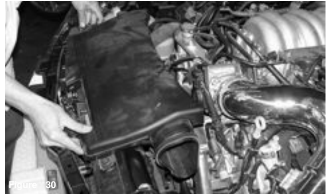
Figure 30 Replace the front air scoop back to its original position once the intake has been installed.
