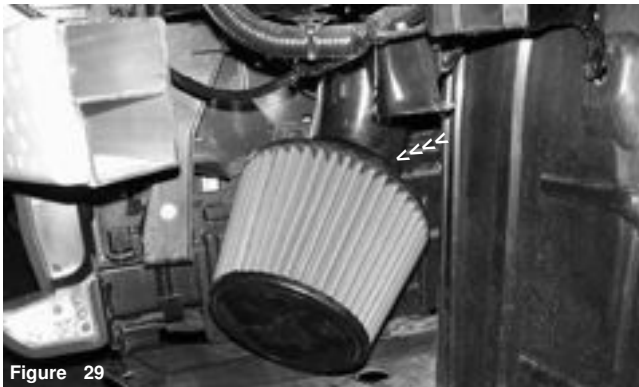
Figure 29 Press the filter over the end of the secondary intake. Once the intake has been butted to the filter stops, continue to tighten the filter neck clamp.
