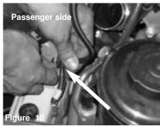
Pull back the engine ground fitting from the bracket located on the passenger side frame of vehicle. This will allow for the installation for the vibra mount.
