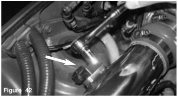
Re-install the temperature sensor and secure using the factory screw. Tighten using 10mm socket and ratchet. *Now install the driver side intercooler pipe and repeat the steps.*
