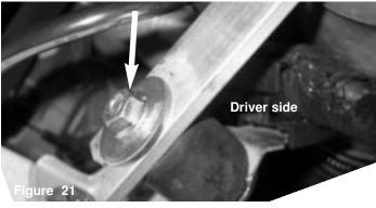
Secure the driver side bracket using provided m6 nut and washer.
