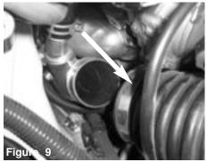
With 8mm nut driver or flat headscrewdriver, loosen the clamp holding in the stock intake tube on the turbo and remove.
