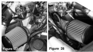
Align the intakes for best possible fit. Once you have aligned and made sure that the length of the intakes are free from any moving parts, continue to tighten all nuts, bolts and clamps.
