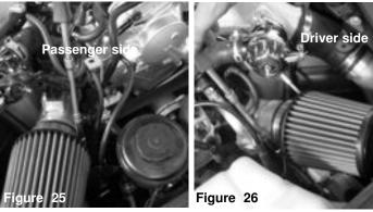
Install filters and secure using 8mm nut driver. Tighten all remaining clamps.
