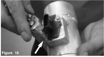
Secure the MAF sensors using the factory screws. Secure and tighten using 7mm socket and ratchet.
