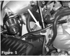
Using a 8mm nut driver, loosen the clamp on the air box. Pull back the intake hose away from the air box.
