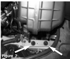
Carefully lift the air box allowing the 2 fitting's on the air box to pull out from the frame of vehicle.
