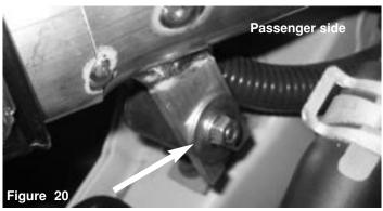
Secure the passenger side tube bracket using provided m6 nut and washer.
