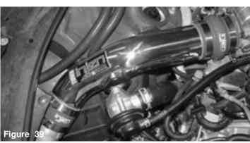
intercooler pipe. Install the 2-3/8" hose to the factory intercooler pipe.
