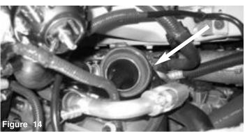
On both sides of the vehicle, install the step hose to turbo with the clamps provided. Position the clamps allowing for easier access. Tighten the clamp on the turbo only.
