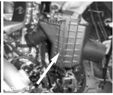
Carefully lift and pull out the air box.
