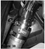
Attach the 2-3/4" hump hose to the new intercooler pipe, intall the intercooler pipe and slide the hump hose on to the throttle body with clamps provided.
