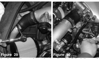
Installation of the upper intercooler pipes, Note: installation is the same for both sides, photos are of passenger side only.
