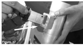
Install the MAF sensors into the correct sideof intake tubes. *NOTE: the driver side tube is longer, passenger tube is shorter.*
