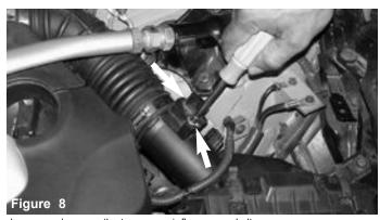
Loosen and remove the two mass air flow sensor bolts.
