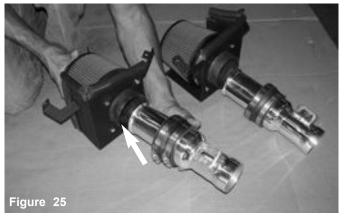
The intake air horns are inserted into the velocity stacks and into the filters. The velocity stack neck should be pressed into the step hose.
