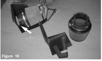
take the assembled filter and velocity stack and insert it into the heat shield opening. Align the nut inseerts to the bolt pattern on the heat shield.
