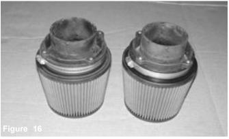
Repeat installation of the second filter and velocity stack. Filters and velocity stacks are now assembled.
