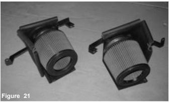
The filters, velocity stacks and heat shields have all been assembled.
