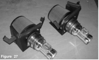
The filters and heat shields have been assembled to the intakes and step
