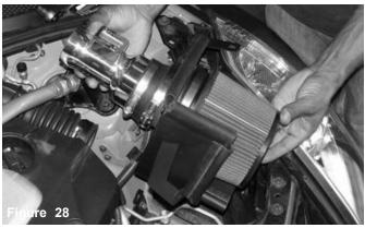
The assembled driver side air filter is now lowered into the driver side engine compartment.
