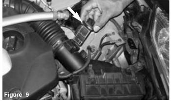
Once you have removed the sensor bolts, continue to pull the mass air flow sensor from the sensor housing.
