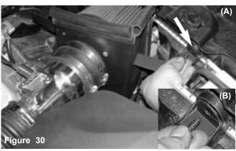
The extended bracket on the heat shield is aligned to the radiator bracket(A), The stock screw is used to secure the bracket to the radiator crossmember(B).
