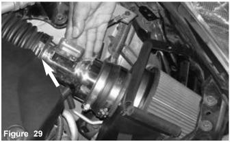
The intake end is inserted into the stock air intake duct. Insert the intake into the air duct until the heat shield brackets are aligned to the mounting holes.
