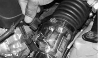
Press the electrical sensor harnes over the mass air flow sensor until it snaps in place.
