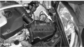
Loosen and remove the 10mm bolt that secures the air box top to the fender.
