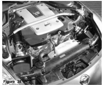
Periodically, check the fitment of both intake systems. Normal driving conditions may loosen nuts, bolts and clamps causing intakes to shift resulting in damage to automotive parts.
