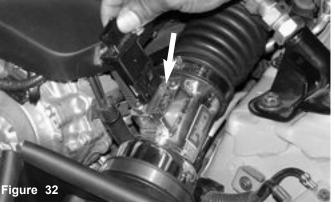
The mass air flow sensor is now inserted into the sensor adapter as shown above.
