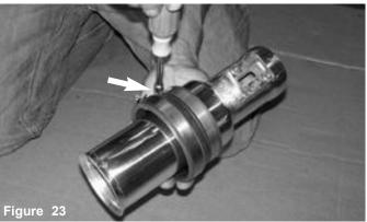
Once you have positioned the step hose in the correct position, continue to tighten the clamp over the intake, repeat install on the second intake.
