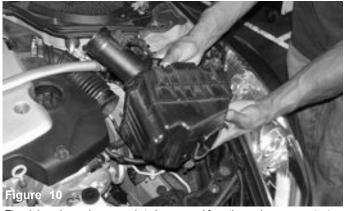
The air box cleaner is now ready to be removed from the engine comparmtnet.
