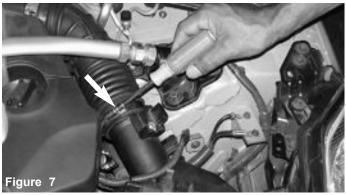
Loosen the air duct clamp that connects the air duct to the sensor housing.
