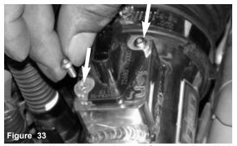
Use two m4  $\,\mathrm{x}\,$  10mm bolts to secure the mass air flow sensor to the machined sensor adapter.
