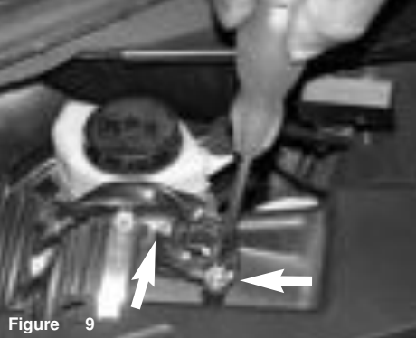
Figure 9 Unscrew the two bolts that secure the mass air flow sensor to the sensor housing.
