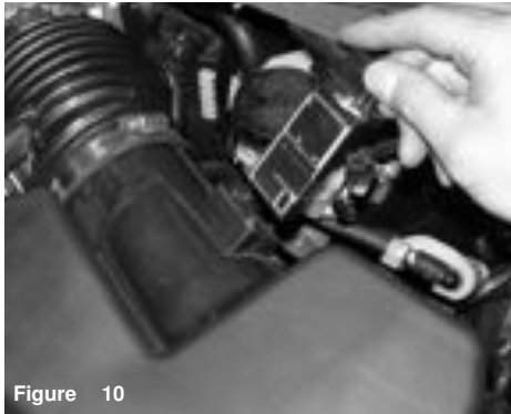
Figure 10 Once you have removed the two bolts, continue to pull the mass air flow sensor out of the sensor housing. This mass air flow sensor will be used later in the installation.
