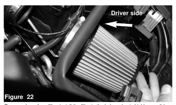
Remove clamp from filter, install the filter to the hole on heat shield, now slide the clamp back on the filter so it sits on the outside. between the shield.
