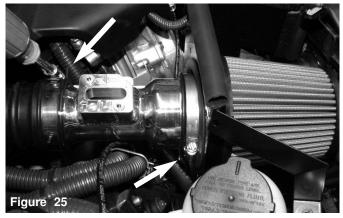
Now install the 2-1/2" side into the factory side of the stock intake tube. Position for the best fit and tighten both clamps using 8mm nut driver.
