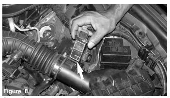
Once you have removed the sensor bolts, continue to pull the mass air flow sensor from the sensor housing.
