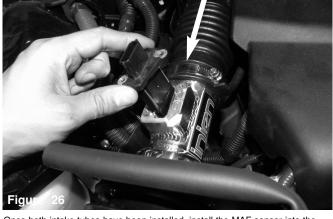
Once both intake tubes have been installed, install the MAF sensor into the intake tubes.
