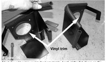
Attach the rubber trim seal to the heat shields. *Look at the list above on the first page for positioning.* Attach the 13" vinyl trim to the inside of the hole cut out on heat shield.
