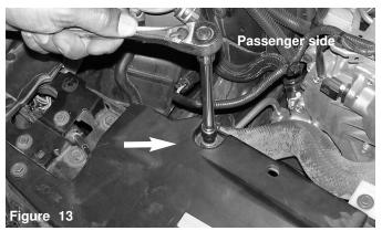
The m6 bolt is loosened from the passenger side shroud as shown above.
