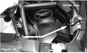
Install driver side heat shield to the vehicle and position. Look back to step 17 for the postioning of the bracket. Secure using the factory screws and tighten.
