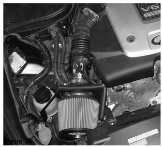
align the passenger side air intake system for the best possible fit. Once the intake and heat shield has been properly adjusted, continue to tighten all nuts, bolts and clamps.
