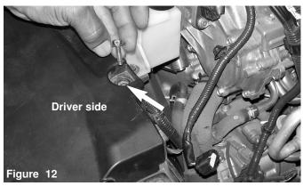
The m6 bolt is now removed from the drive side shroud to be used later in the instructions.
