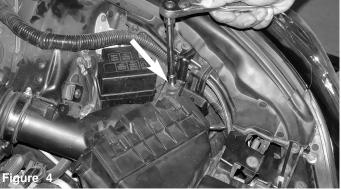
Loosen and remove the 10mm bolt that secures the air box top to the fender.
