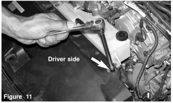
The m6 bolt is Loosened from the driver side shroud as shown above.
