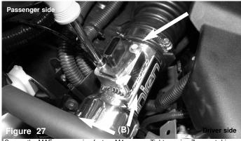
Secure the MAF sensor using factory M4 screws. Tighten using 7mm nut driver.
