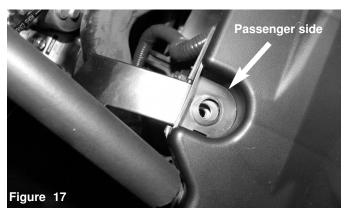
Install the passenger heat shield to the vehicle and position the bracket under the plastic from step 13. Now secure using the factory bolt. *Note: also repeat on the driver side heat shield install.*
