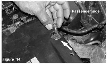
The m6 bolt is now removed from the passenger side shroud to be used later in the instructions.
