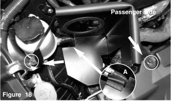
Secure the heat shield using the screw from step 4. Tighten both screws using 10mm socket and ratchet. A) Attach the 1-1/2" rubber trim to the shield if the factory hose is close to the shield.
