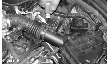
Loosen the air duct clamp that connects the air duct to the sensor housing.
