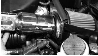
Install the intake tubes into the vehicle, hold filter and refer back to steps 20&21 for positioning. Position the MAF pad facing up.
