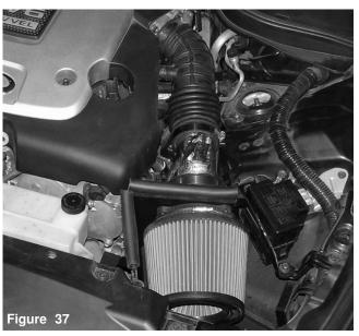
align the driver side air intake system for the best possible fit. Once the intake and heat shield has been properly adjusted, continue to tighten all nuts, bolts and clamps.
