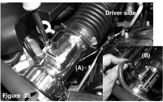
A) Continue to driver side and make secure. B) Re-connect both MAFsensor Harness'.
