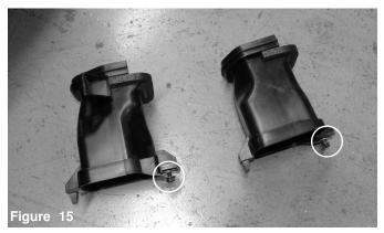
Optional is the removal of the factory snorkels. A 10mm screw is holding them in each on the radiator support.
