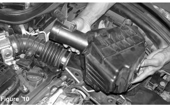
The air box cleaner is now ready to be removed from the engine compartment.
