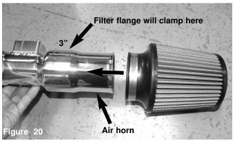
Do not install. The intake tube contains air horn. The filter will slide on to the intake tube past the air horn and clamp on the 3" section of the tube.
