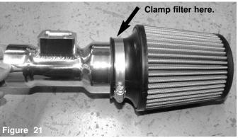
Do not Install. Make sure the the filter sits past the air horn. Once the filter slides past the air horn, (may require light force) filter will hit a stop, now position and tighten.
