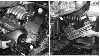
You are now ready to remove the entire air intake box and air intake duct from the engine compartment (A). Once the bumper has been removed continue to remove the air intake resonator from the drive side bumper (B).
