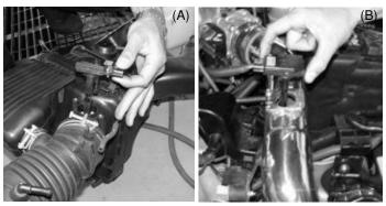
Remove the mass air sensor from the stock air intake box (A). Carefully place the mass air sensor into the machined flange welded to the intake (B). Use the stock screws to fasten the sensor to the machined flange.
