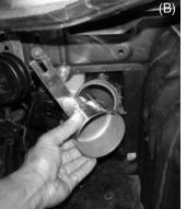
Take the medium clamp and locate it over the end of the silicone intake (A). Take the coupler with bracket and press it into the silicone intake (B).
