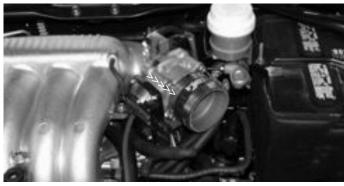
Take the  $2\ 3/4$ " straight hose and press it over the throttle body, use two clamps and tighten the clamp on the throttle body side.
