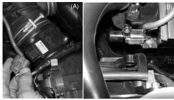
Disconnect the mass air sensor harness (A). Disconnect the plug connected to the vacuum switching valve (B).
