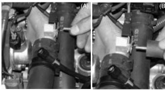
Remove the m6 bolt screwed into the thermostat housing(A) Now take the m6 vibra-mount and screw it into the pre-tapped hole as shown above (B).
