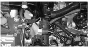
The vibra-mount is shown fully screwed into the thermostat housing.
