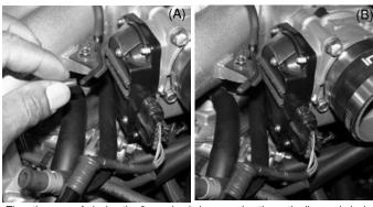
The other way of placing the 3mm plug is by removing the entire line and placing the 3mm plug over the port and shown in (A) and (B).
