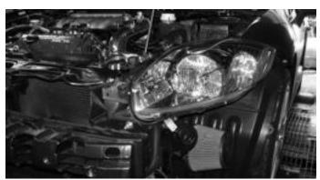
Once the entire cold air intake has been installed, adjust for best possible fit. Once the intake has been cleared from rubbing and rattling continue to tighten all nuts, bolts and clamps. Periodically, check for rubbing, leaks or rattling along the length of the intake in order to avoid damage to the intake.
