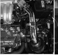
The short ram installation is now complete (A). Installation of the cold air intakelocate the remaining vibra-mount and screw it into the pre-tapped hole located on the side of the main frame (B).
