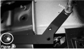
Once the first m8 bolt is semi-tightened as circled above, continue to align the second m8 x  $21\,\text{mm}$  bolt to the car frame.
