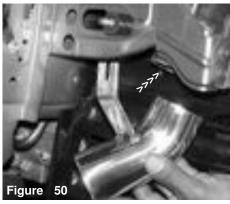
Align the extended intake to the secondary silicone hose as shown above.
