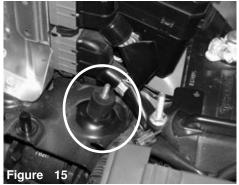
The m6 vibra-mount is sitting flush over the air box mounting plate.
