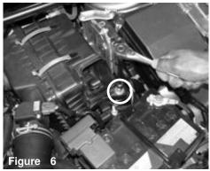
Unscrew the air box cleaner m6 bolt from the brace.
