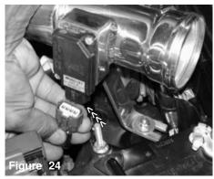
Press the electrical sensor harness clip over the mass air flow sensor until you hear them snap together.
