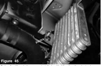
Both m8 x 16mm bolts are now installed and holding the oil cooler in place.
