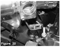
The intake bracket is sitting flush over the vibramount stud.
