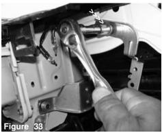
The m8 bolt holding the upper brace is loosened and removed.
