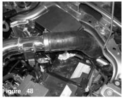
The upper silicone hose is pressed over the primary intake.
