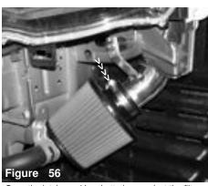
Once the intake end has butted up against the filter stops, continue to tighten the filter neck clamp.
