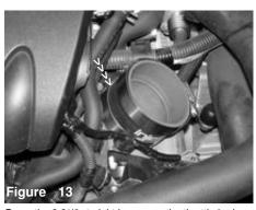
Press the 2 3/4" straight hose over the throttle body. Slip two power-bands over the 2 3/4" hose and tighten the clamp over the throttle body.
