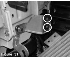
The two m8 bolts fastened to the zinc plated brace have been loosened and removed. The oil cooler is now detached from the brace.
