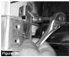
The final two m8 bolts are removed from the larger zinc plated brace that is attached to the car frame.
