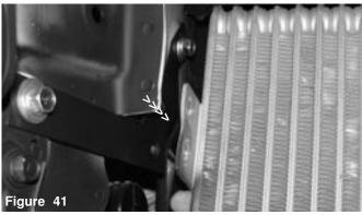
The oil cooler is now aligned to the new bracket as shown above.
