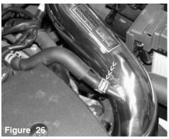
Once you have pressed the breather hose over the intake air port, continue to use the tension clamp over the breather hose. All non-GTS models, proceed and go to figure 46 to continue.
