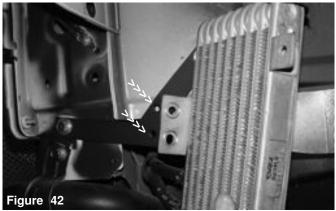
The oil cooler brace is aligned to the press nuts located on the bracket.
