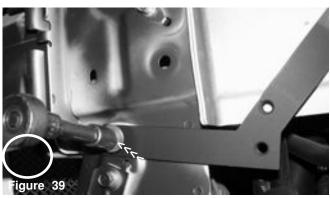
The first m8  $\times$  21mm bolt is aligned to the frame to  $\,$  fastened the new bracket.
