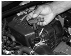
Once the m4 bolts have been removed, continue to pull the mass air flow sensor from the sensor housing.
