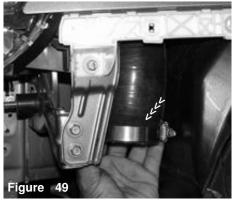
Slip one power-band over the end of the secondary silicone.
