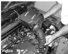
Now the all nuts, bolts and clamps have been removed or loosened, continue to pull the air box cleaner from the engine compartment.
