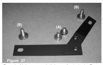
The stock m8 bolts are now used with the new oil cooler bracket. The two m8 x 16mm bolts (A) are fastened to the press nuts while the two m8 x 21mm bolts (B) are used to attach the entire bracket to the car frame.
