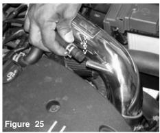
The stock crank case breather hose is now aligned to the intake port as shown above.
