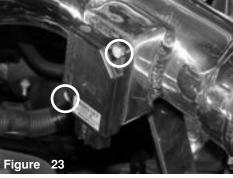
Use the m4 bolts provided in this kit to fasten the mass air flow sensor to the sensor adapter.
