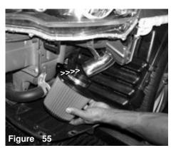
Align and press the filter neck over the intake end.
