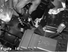
Align the m6 vibra-mount over the air box mounting point as shown above.
