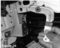
The L-shape zinc plated brace is now removed from the top frame.
