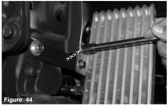
The second m8  $\times$  16mm bolt is aligned and fastened to the upper press nut.
