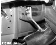
Use the m6 flange nut and fender washer to fasten the intake bracket to the vibra-mount stud.
