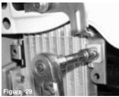
The first m8 bolt is loosened and removed.
