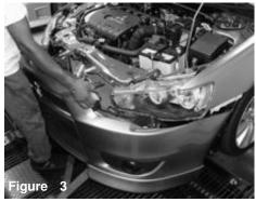
the front bumper in place, continue to remove the front front air scoop. bumper as shown above.
