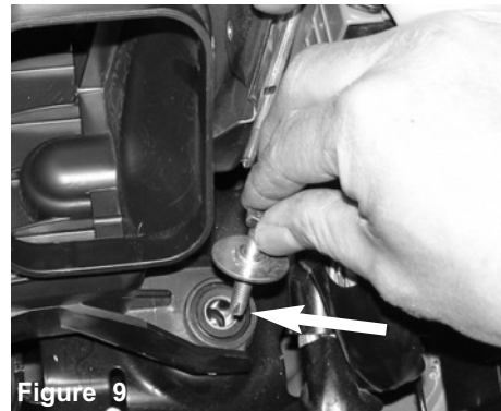
Figure 9 Once you have loosened the m6 bolt, continue to pull the m6 bolt out.
