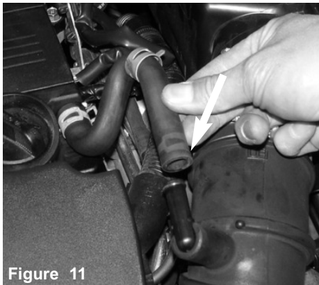
Figure 11 Once the tension clamp as been pulled back, pull the crankcase vacuum hose from the air duct port.
