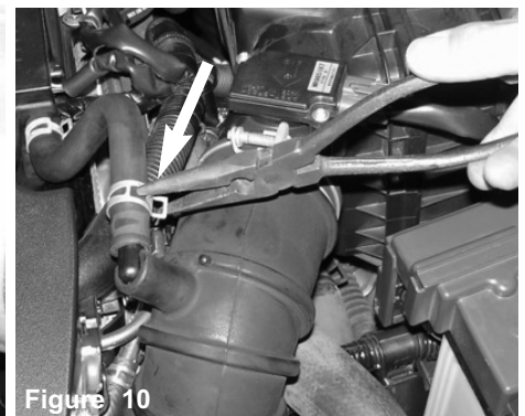
Figure 10 The tension clamp is compressed and pulled from the crank case vacuum hose located over the air intake duct.
