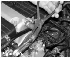
Use a pair of pliers to depress the tabs on the breather hose tension clamp. Pull the tension clamp away from the PCV pipe.
