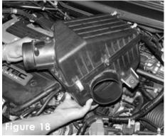
Once you have removed the three bolts, continue to pull the air box cleaner out of the engine compartment
