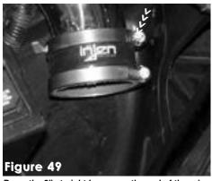
Press the 3" straight hose over the end of the primary intake, use the power-bands on the hose and fasten the clamp over the primary intake.
