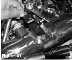
Press the electrical harness clip over the mass air flow sensor until it snaps in place.
