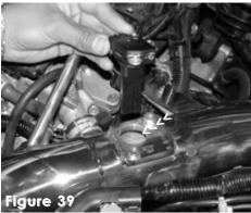
Insert the mass air flow sensor into the machined sensor adapter. Rub a dab of light oil on the Oring, this will avoid kinking of the O-ring.
