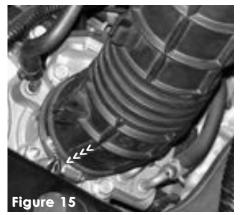
Loosen the clamp on the air intake duct connected to the throttle body.
