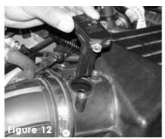
Once you have removed both bolts, continue to pull the mass air flow sensor from the sensor housing.
