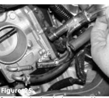
Once the tension clamp has been removed from the upper coolant idle port, continue to pull the hose from the coolant idle port.
