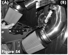
Align the filter to the intake end (A). The filter is pressed over the intake until the intake is butted up against the filter stop. Tighten the filter clamp located on the filter neck (B).
