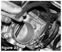
The 12"-8mm heater hose is pressed over the upper coolant idle port. The stock tension clamp is used to secure the 8mm heater hose in place.
