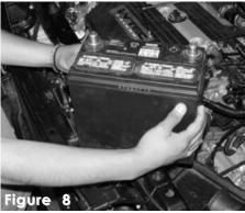
With the battery tie down out, continue to remove the battery from the engine compartment.
