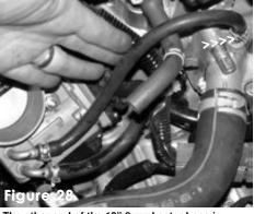
The other end of the 12" 8mm heater hose is pressed over the coolant outlet port. The tension clamp is used to secure the hose in place.
