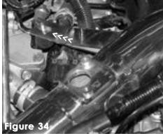
The intake bracket is aligned to the vibra-mount stud.
