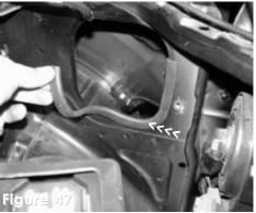
Press the 12" vinyl trim along the edge of the fender well resonator opening.
