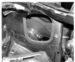
The vinyl trim is flush around the fender well resonator opening.
