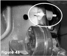
The m6 flange nut and fender washer is used to secure the vibra-mount over the horn bracket.
