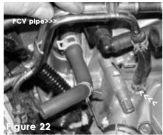
The tension clamp is depressed on the coolant outlet hose and pulled back.
