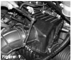
Loosen the air intake duct clamp from the air box cleaner.
