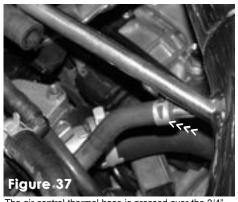
The air control thermal hose is pressed over the 3/4" shorter intake port, the stock tension clamp is used to secure the hose in place.
