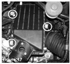
Use a 10mm socket and ratchet to loosen and remove all three bolts from the air intake box.
