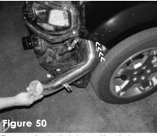
The secondary intake is inserted into the bumper area and into the fender well resonator opening.
