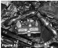
Align the intake for the best possible fit. Once you have aligned the entire intake, continue to tighten all nuts, bolts and clamps.
