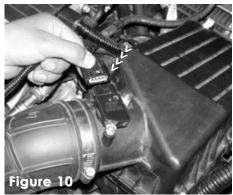
Disconnect the electrical harness clip from the mass air flow sensor.
