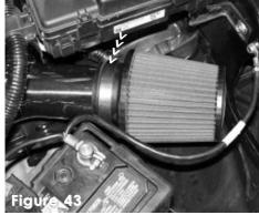
Press the intake end into the filter neck until it butts up against the filter stops. Tighten the filter clamp once the filter is flush with the intake.
