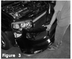
Remove all top plastic clips, bottom and side screws, then continue to pull the front bumper away from the front end. Set the bumper down on the floor once you have pulled it away from the front end.
