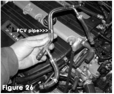
The PCV pipe and coolant hoses are now removed from the engine compartment.
