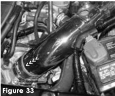
Insert the intake into the throttle body hose until it sits flush with the throttle body edge.
