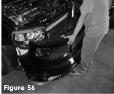
Continue to reinstall the battery and battery tie down. Replace the front bumper back to its original position and use the stock pins and screws to secure the bumper.
