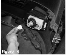
With the bumper sitting on the floor continue to disconnect the fog lamp electrical harness clips as shown above.
