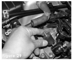
Align and screw the vibra-mount to the air box cleaner bracket.
