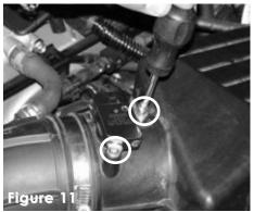
Loosen and remove both sensor bolts from the mass air flow sensor.
