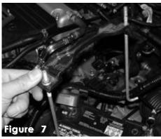
Once you have loosened both nuts, continue to remove the battery tie down as shown above.
