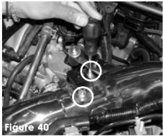
The stock bolts are used to fasten the mass air flow sensor over the machined adapter.
