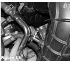
The air control thermal hose is disconnected from the port on the air intake duct.
