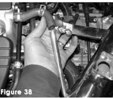
Press the long 3/8" intake port into the crankcase breather hose as shown above. Use the stock tension clamp to secure the breather hose in place.
