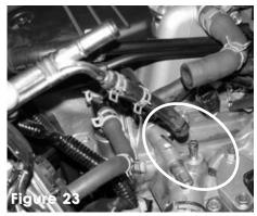
With the tension clamp pulled back, continue to pull the coolant outlet hose from the port.
