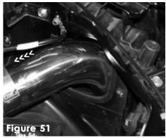
The secondary intake is pushed through the fender well resonator opening. The top end is inserted into the primary intake.
