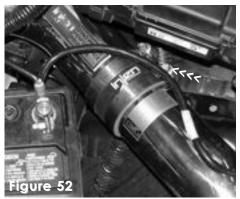
The secondary intake is pressed into the hose located on the end of the primary intake. Once the intake is aligned, continue to fasten the power-band
