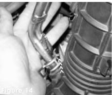
Press the tension clamp tabs together and gently pull the clamp away from the air intake port.
