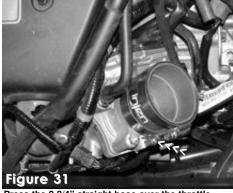
Press the 2 3/4" straight hose over the throttle body until it is butted up against the end. Tighten the power-band to over the throttle body to secure hose over the throttle body.
