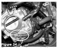
The tension clamp on the upper coolant idle port is depressed and moved back.
