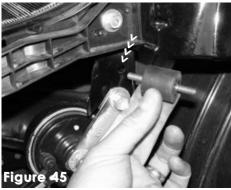
The secondary vibra-mount is aligned above the horn bracket.
