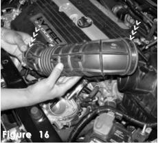
Now that all clamps on the air intake duct are loosened, continue to remove the air duct from the throttle body and air box cleaner.
