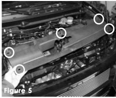
Remove all five plastic clips from the plastic shroud and remove the shroud from the radiator and cross member.
