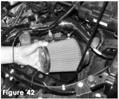
You can temporarily convert to a short ram during heavr rain fall but this intake system has been tuned for cold air configuration.
