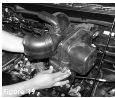
Now that the air box cleaner is out of the engine compartment, continue to pull the resonator box from the fender well.
