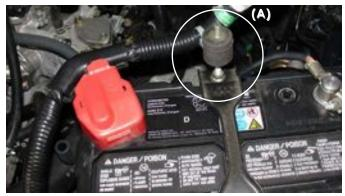
Screw the female vibra-mount over the battery post (A),  $\,$  Usually,  $\,$  8 complete turns will be enough to level the intake bracket.
