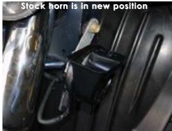
The screw is tightened into the bumper frame and the horn is now relocated.
