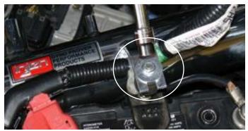
Place the m6 flange nut and fender washer over the intake bracket and vibramount stud. Take the m8 socket and Ratchet and semi-tighten the flange nut for
