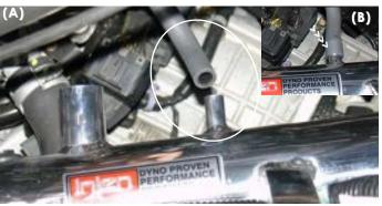
Insert the stock 8mm hose over the 3/8" intake port (A). Press the breather line just enough to hold itself in place (B).
