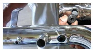
Take the 1525 sensor grommet at place it into the 3/4" pre-drilled hole (A). The sensor grommet groove will fit snug around the 3/4" holes edge (B).
