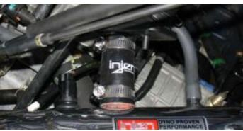
Here, the air temperature sensor, CCV hose, CCV box, and breather lines have been installed and completed.
