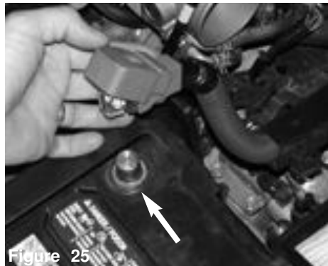
Figure 24 Disconnect the negative battery terminal
