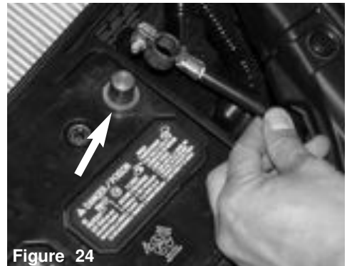
Figure 25 Now disconnect the positive battery terminal.
