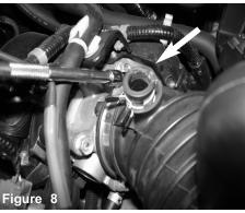
Loosen the clamp on the throttle body using 8mm nut driver.
