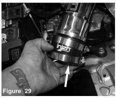
Remove the filter and install to the upper intake tube assembly.
