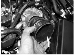
With clamps provided, install the 2-7/8" hose to the throttle body.
