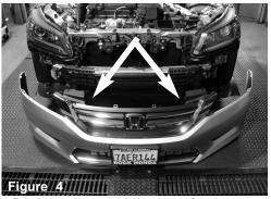
Front bumper cover needs to be removed from the vehicle for the factory resonator to be removed. Remove the plastic push-clips from top and bottom and remove side screws from the splash guard. Carefully pull back bumper cover. Disconnect Fog lights if equipped.
