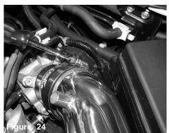
Tighten the clamp on throttle body using 8mm nut driver
