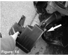
Remove the resonator from vehicle, this may require some force to push down and away from vehicle.
