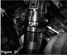
Secure and tighten the clamps on filter.
