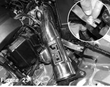
Install the upper intake tube to vehicle and position the bracket to the vibramount. Secure and tighten using provided M6 nut and fender washer.
