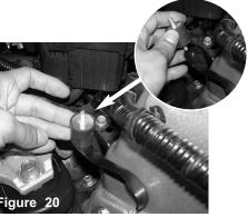
Now install the vibra mount to the bracket using original airbox location.
