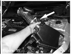
Disconnect the harness that is attached to the base of the air box near throttle body. Now lift up and remove the air box from the vehicle.
