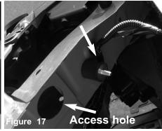
Now install the provided M6 vibra mount. Secure and tighten.
