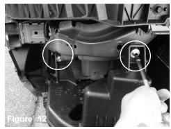
Loosen the 2 bolts holding in the resonator box.
