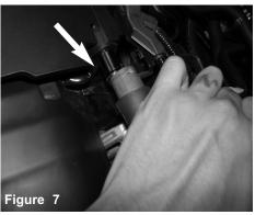
Pull the crank case line away from the engine fitting.
