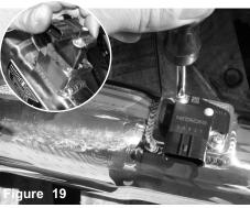
Now install the sensor into the intake tube, secure and tighten using factory screws from previous step.
