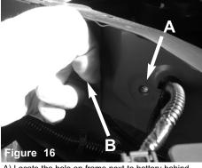
A) Locate the hole on frame next to battery behind headlight B) Now use larger hole to slide inside the washer and M6 nut and line up to hole( see figure 17 for photo of hole).
