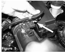
Disconnect the MAF sensor harness and pull the line away from the air box.
