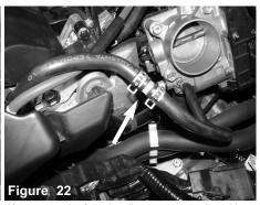
Now secure the 2 coolant lines together using white nylon coupler. Secure using factory clamps.
