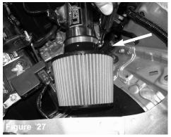
Install the filter to the upper intake tube and tighten using 8mm nut driver.
