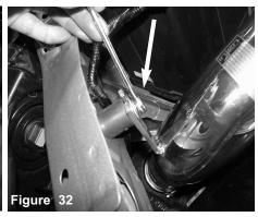
Secure the vibramount using provided m6 fender washer and nut. Install the filter to the lower intake assembly and tighten using 8mm nut driver.
