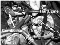
NOTE:Make sure vehicle is cool before performing this step. Remove the hard line/crankcase line from vehicle. Disconnect the crankcase side from the engine side. Remove both coolant hoses from the hard line.
