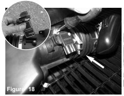
Loosen the 2 screws holding in the MAF sensor using phillips screwdriver and remove the sensor. Save the screws for later install.
