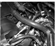
Install provided 15mm hose to the engine and intake tube fittings.
