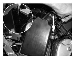
With 10mm socket and extension, loosen the 2 screws Pull back the intake tube from the throttle body. holding in the air box.
