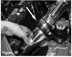
Now install the lower intake assembly into vehicle.
